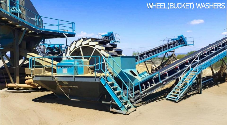
**CONSTMACH Wheel Washers** are designed for washing out the clay in the sand for the purpose of increasing the sand quality. Thanks to their simple design they have an ease in assembly process. These bucket wheels provide advantages to the users with low power consumption and water saving.
