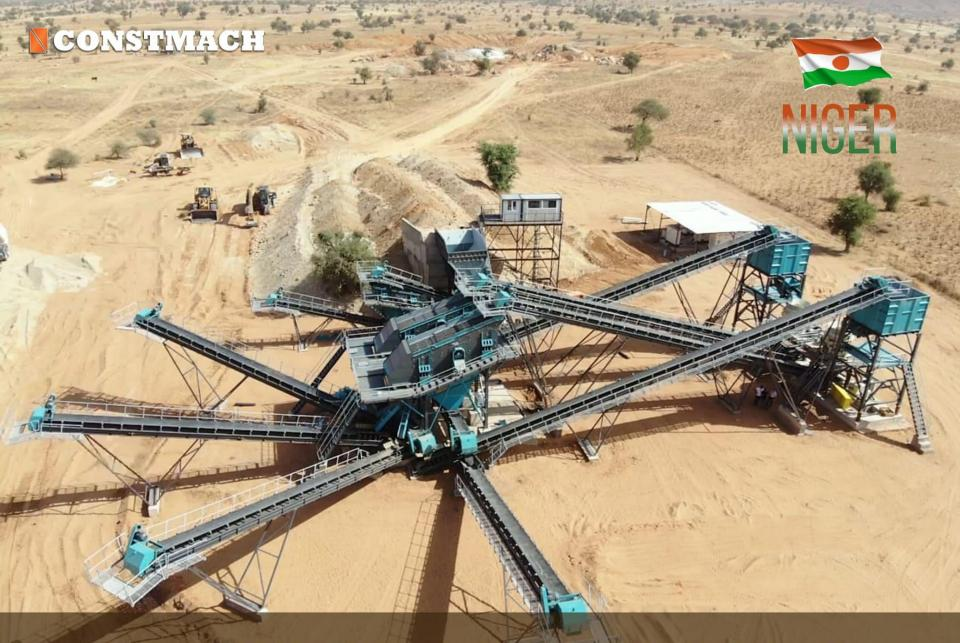
FIX JCC - 3 / STATIONARY CRUSHING AND SCREENING PLANT
