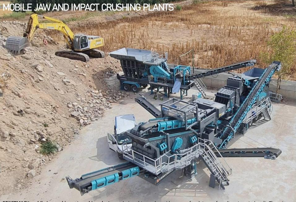
**CONSTMACH mobile jaw and impact crushing plants** are designed to crush a wide range of rock types, from limestone to basalt. The primary jaw crusher efficiently processes large and hard rocks, while the secondary impact crusher ensures the production of well-shaped, cubic final materials. Depending on customer requirements, the final output size can range from **0 to 60 mm**.
