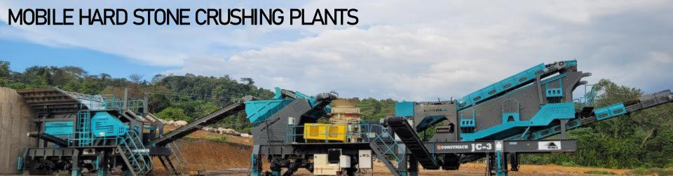
A mobile hard stone crusher is the perfect solution for crushing extremely hard rocks with high abrasiveness and a high silica (SiO<sub>2</sub>) content, such as granite, basalt, and gabbro. The primary jaw crusher enables the processing of large and hard rocks, while the secondary cone crusher ensures efficient second-stage crushing of even the toughest materials.
