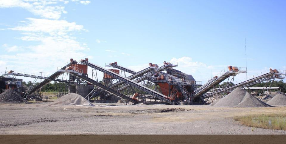
FIX JCV - 3 / STATIONARY CRUSHING AND SCREENING PLANT
