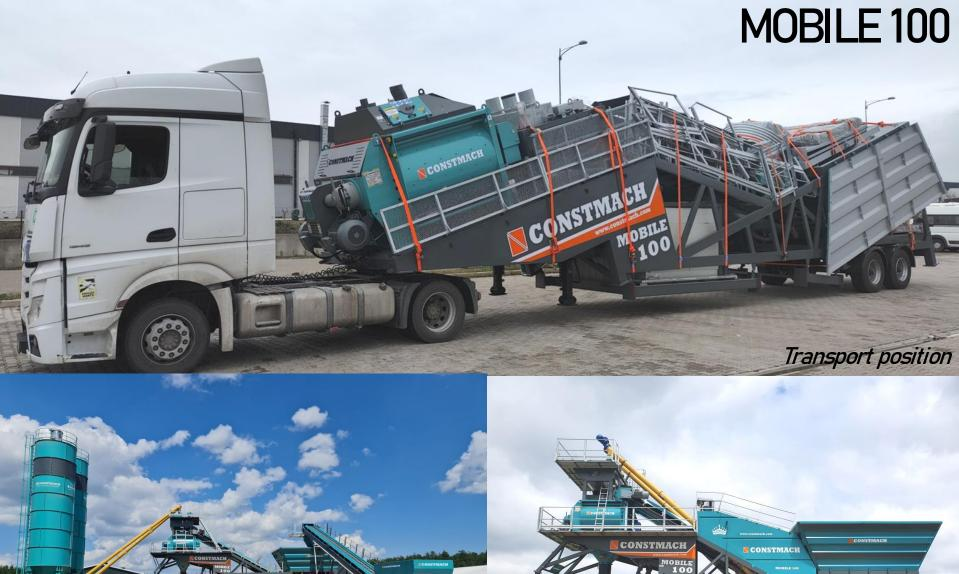
With external cement silo and pre-feeder
